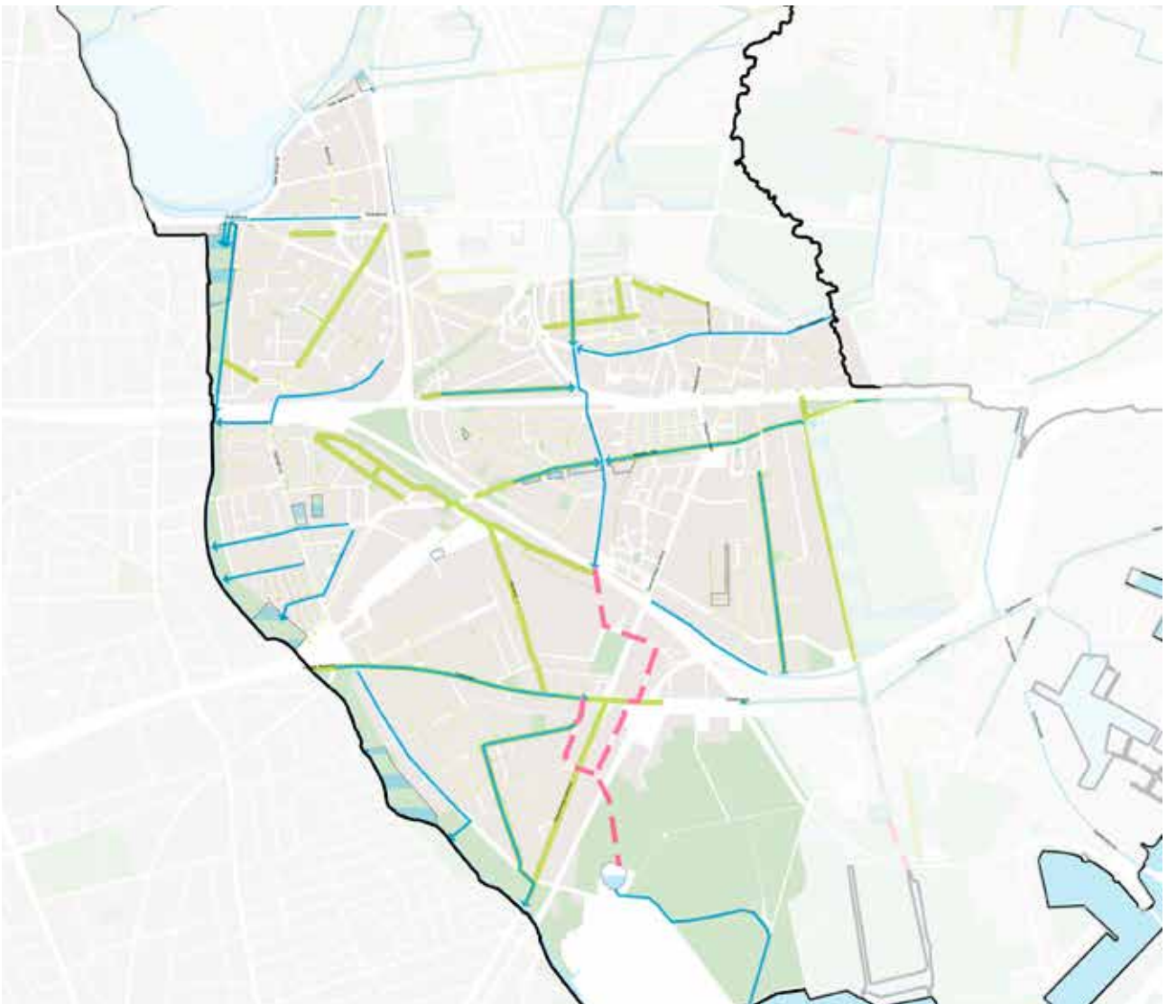
Valby with water catchment areas and cloudburst management projects
