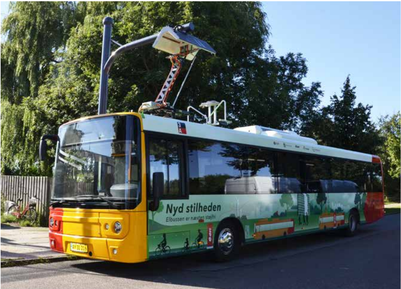
The pole-mounted charging stations are especially designed for city use, and can recharge the bus in 1-3 minutes. Photo by City of Copenhagen
