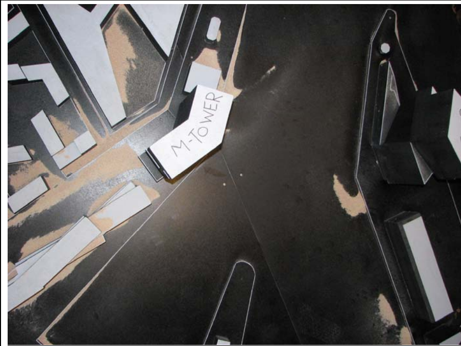
M-Tower Wind Speed = 9.0 m/s
