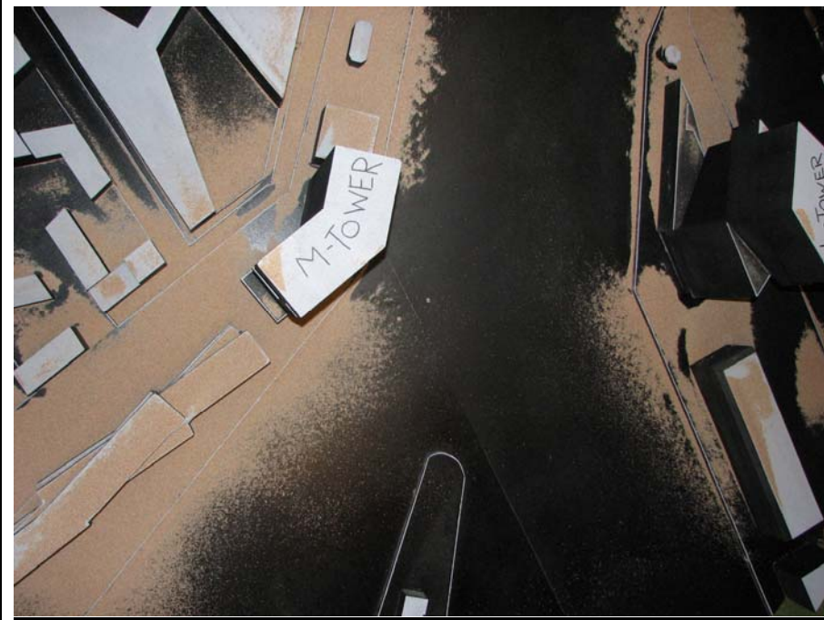
M-Tower Wind Speed = 4.5 m/s
